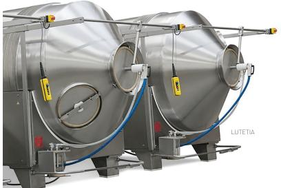
Patented and innovative technologies for healthier products: Lutetia R&D team has developed large, industrial solutions to efficiently meet the requirements of low salt and clean label products.
